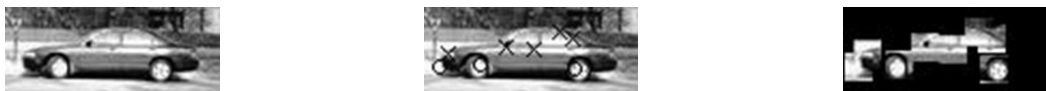
Fig. 1. Left: A sample object image used in vocabulary construction. Center: Interest points detected by the F o rstner operator. Crosses denote intersection points; circles denote centers of circular patterns. Right: Patches extracted around the interest points
